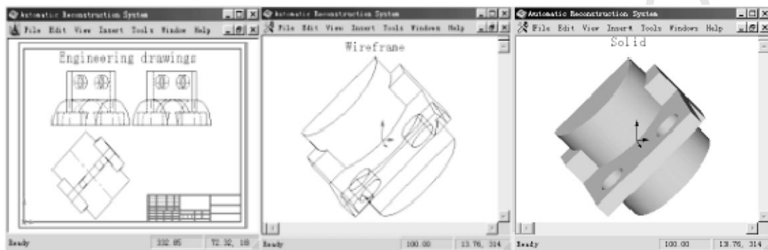
Fig. 14. Engineering drawings and reconstructed model for object 3.
