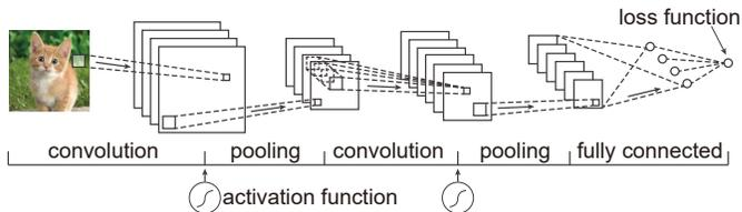
Fig. 2. The typical architecture of a CNN.
