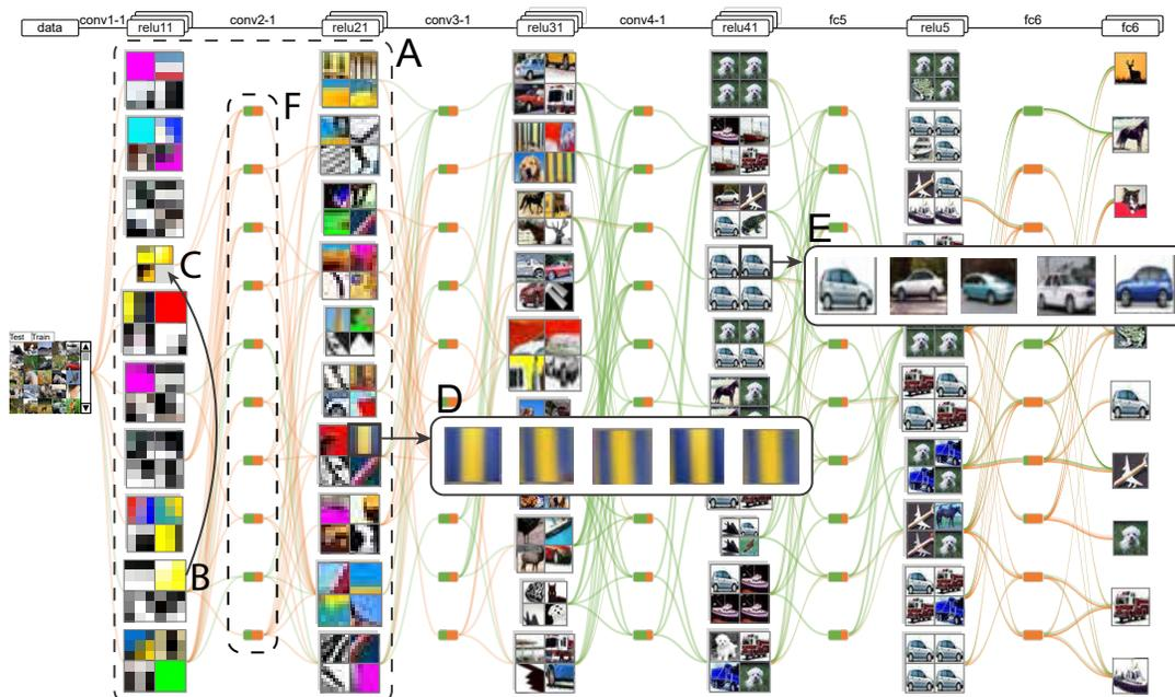
Fig. 1. CNNVis, a visual analytics system that helps experts understand, diagnose, and refine deep CNNs.
