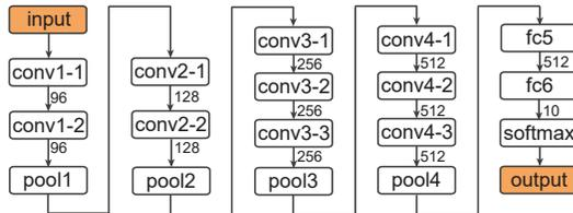
Fig. 9. The architecture of BaseCNN. It contains four groups of convolutional layers and two fully connected layers. The number below a layer is the number of neurons in that layer.
