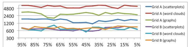
Fig. 10. Time (measured in milliseconds) needed for resizing different visualizations using the adaptive grid (Grid A) and the significance-aware grid (Grid B).
